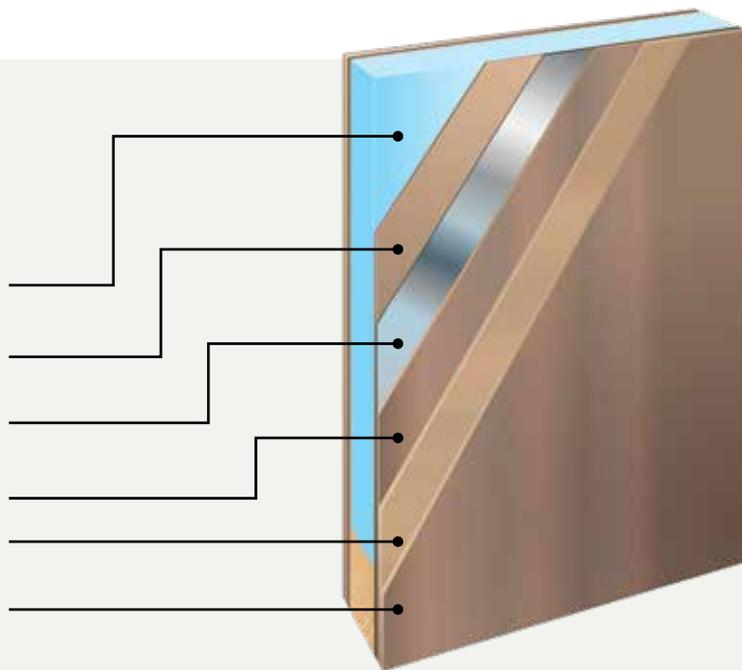
The composite door has a bonded sandwich construction providing a high degree of stability, with the aluminium plates acting as an effective moisture barrier.
